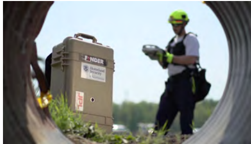
The suitcase-sized FINDER can locate surviving victims buried under feet of rubble in disaster areas. Courtesy of NASA/JPL-Caltech/DHS
