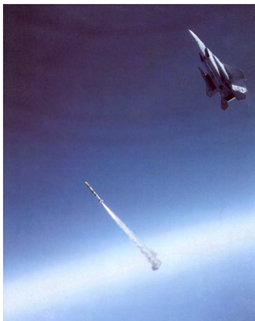
U.S. F-15 Eagle jet fighter fires an ASM-135 missile to destroy a satellite. Courtesy of USAF, Photo by Paul Reynolds
