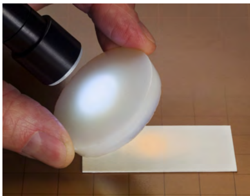
Aerogel, one of the lightest solid materials known, is also an excellent insulator. Courtesy of NASA
